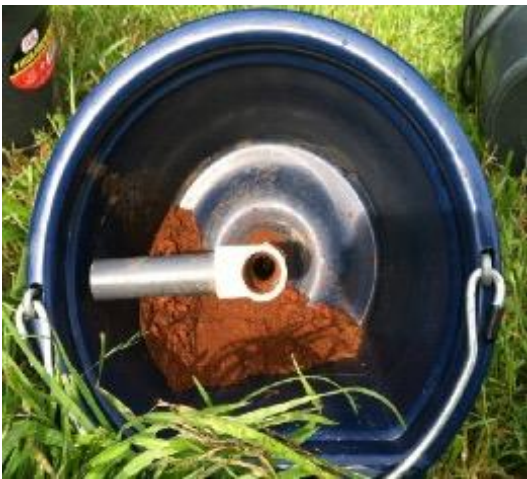
Figure 9. Image showing the soil buildup inside the pipe in the client's tee-bar style unit, using a 5/8-inch Long Ship Auger drill bit and 3/4-inch Schedule 80 PVC pipe. Excessive wall-to-bit clearance was a factor. Photo credit: W. Bryan Smith, Clemson University.
