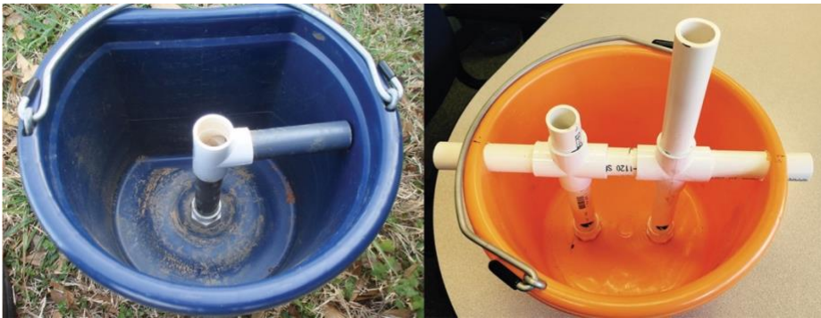
Figure 6. Client modifications to prevent PVC pipe from spinning when sampling moist soils. The side handle is held while sampling (image on left). This design has multiple soil exit holes. Photo Credit: Reed Edwards, Laurens County Cattleman. Another design has two sampling depths and pipe through the pail sides for stability (image on right). This design has single soil exit holes. Photo credit: RD Morrison, Oconee County Cattleman and Lindsey Craig, Clemson Extension Service Livestock and Forages Agent.
