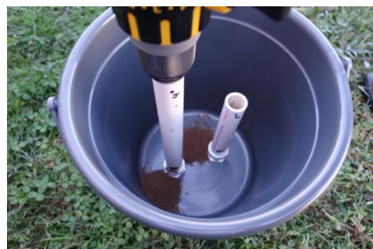
Figure 4. The completed original single-hole unit in operation, showing dry soil exiting the pipe from the holes on both sides of the PVC pipe. Photo credit: W. Bryan Smith, Clemson University.
