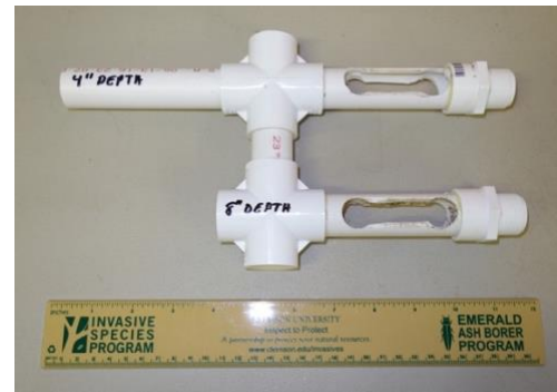
Figure 8. A completed long hole two-depth pipe assembly ready to be inserted in the pail with crosses in place in case torque on the PVC pipe occurs. Note the labels on each pipe noting the soil sampling depth. Photo credit: W. Bryan Smith, Clemson University.
