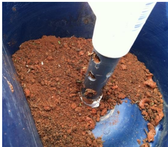
Figure 10. Even with multiple soil outlet holes, this design showed plugging issues in the 3/4-inch Schedule 80 PVC pipe, which possibly also contributed to the soil layer deposit in the pipe. Photo credit: W. Bryan Smith, Clemson University.
