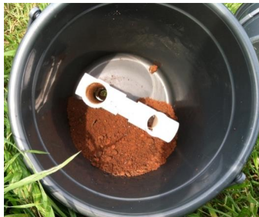
Figure 12. Both units were used to sample an equivalent number of soil cores. This design not only showed no torque force on the pipe, but also showed little sign of soil buildup inside the pipe. Photo credit: W. Bryan Smith, Clemson University.
