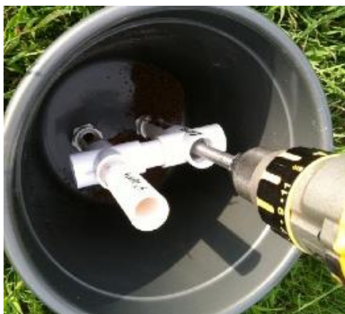
Figure 11. The long hole exit unit in use. This unit has two pipes to allow both 4-inch and 8-inch-deep soil sampling. Note the soil exit holes are facing the pail sides, not the adjacent pipe, to prevent soil loss through the pipe not being used. Photo credit: W. Bryan Smith, Clemson University.
