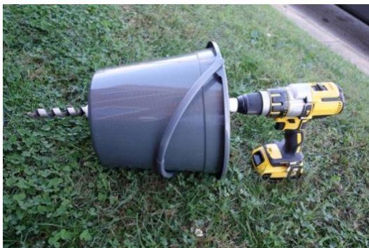
Figure 5. Figure 4. Completed unit showing the drill bit extending four inches past the male adapter after the drill chuck comes in contact with the PVC pipe. Photo credit: W. Bryan Smith, Clemson University.
