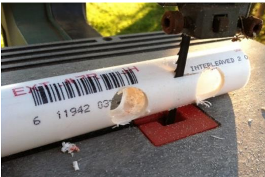
Figure 7. Two 3/4-inch holes were drilled in the pipe with a hole saw. A band saw was then used to remove material between the holes drilled to provide a larger soil exit point. Photo credit: W. Bryan Smith, Clemson University.
