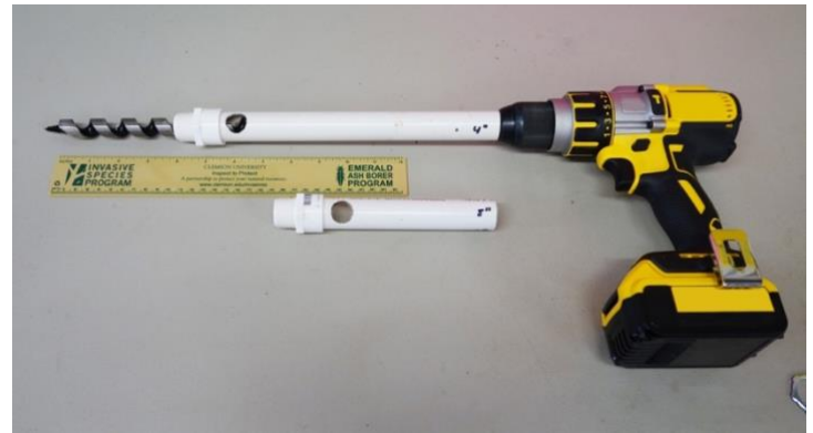
Figure 2. Completed PVC pipes used in the first design to limit sampling depth (one 4-inch depth; one 8-inch depth). Note the single hole which will allow soil to exit into the pail when installed. Photo credit: W. Bryan Smith, Clemson University.
