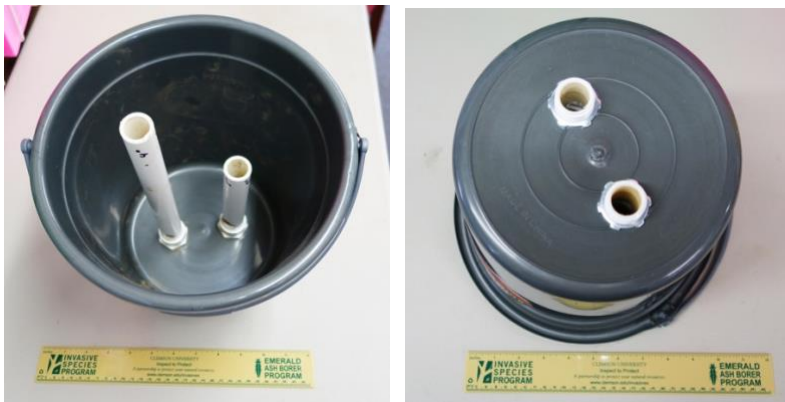
Figure 3. Completed Modified Sweatless Soil Sampler with single exit hole in the PVC pipes. This model has two sampling tubes installed, one for a 4-inch sampling depth and another for an 8-inch sampling depth. Note the conduit nuts on the bottom of the pail holding the male adapters in place. Photo credit: W. Bryan Smith, Clemson University.
